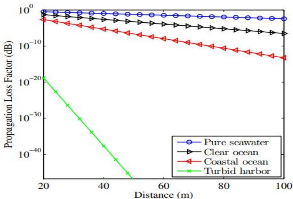
Fig. 3. Attenuation of the optical signal [6]
