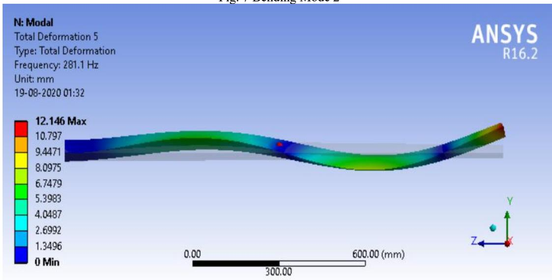
Fig. 8 Bending Mode 3
