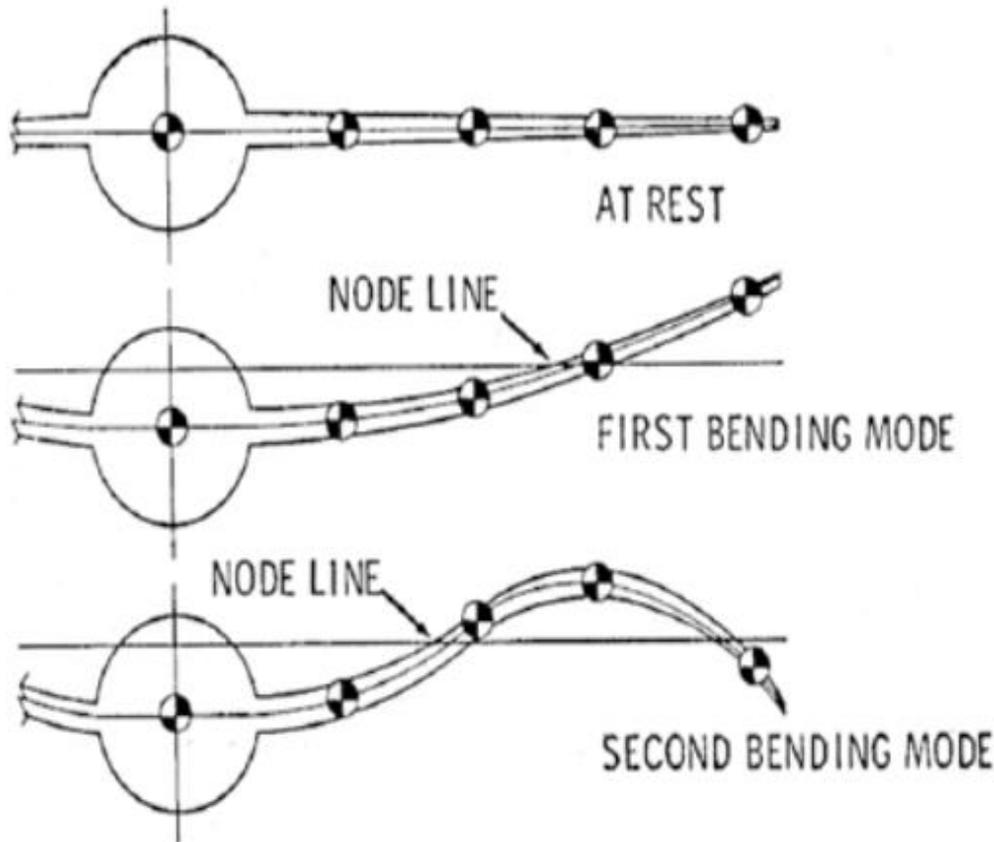
Fig. 1 Mode shapes in an aircraft wing
