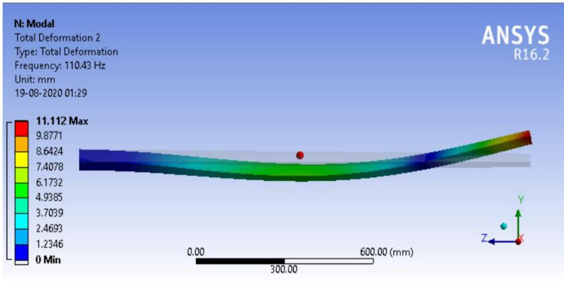
Fig. 7 Bending Mode 2
