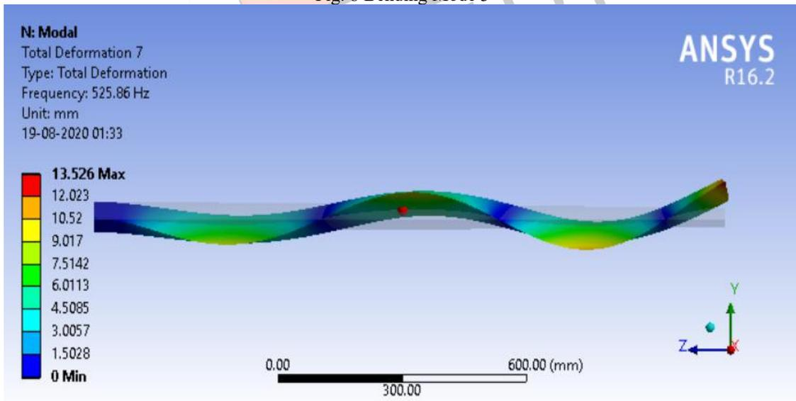
Fig. 9 Bending Mode 4
