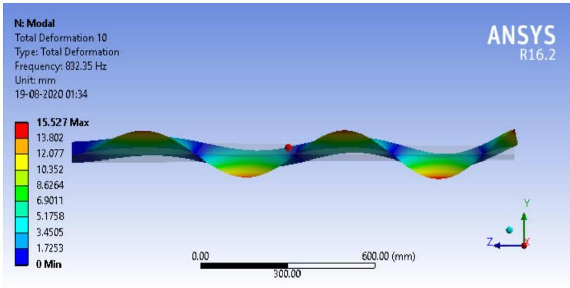
Fig. 10 Bending Mode 5
