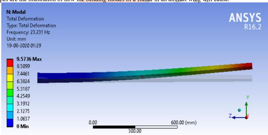
Fig. 6 Bending Mode 1
