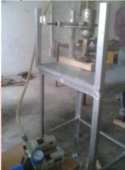
Fig 2 : Fabricated Experimental Setup of Abrasive jet Machining
