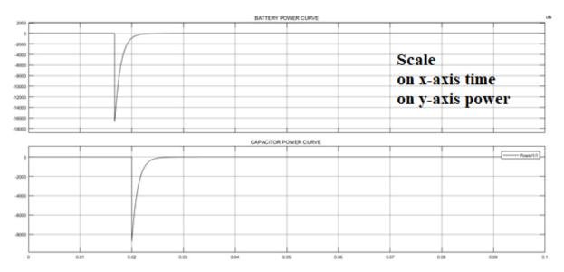
Fig. 8 Power curves of battery and super capacitor
