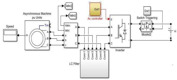
Fig. 3 Simulink model of VSG
