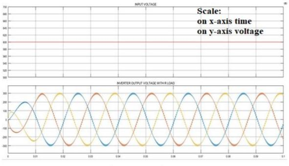
Fig. 6 Input and Output values of VSG
