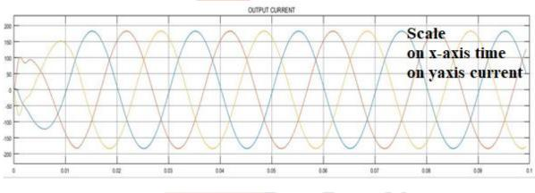
Fig. 7 Output current of VSG
