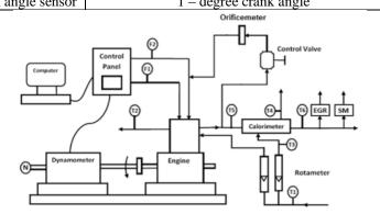
Fig -1: Experimental setup with EGR
