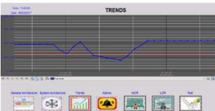
Fig 7: Trends of Solar SCADA
