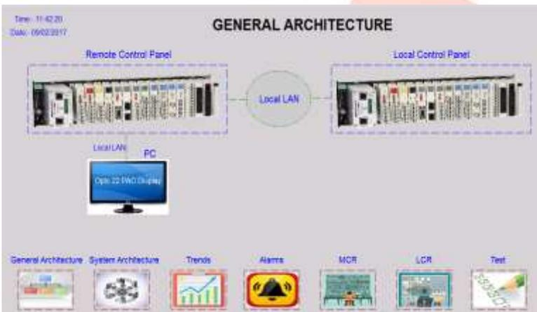
Fig 6: PAC Display General Architecture of Solar SCADA
