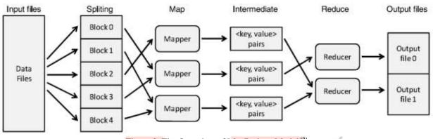
Figure 2. The Overview of MapReduce Model<sup>[2]</sup>
