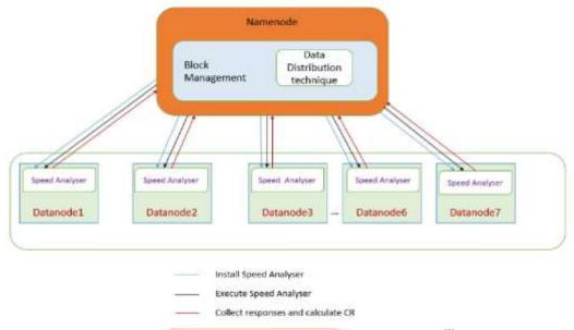
Figure 4. Proposed Data-Distribution Architecture<sup>[3]</sup>
