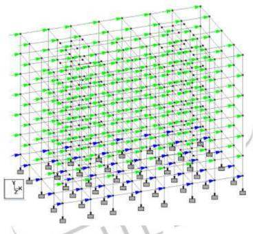
Earthquake Load in Z-direction
