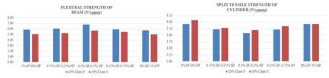
Split Tensile Strength Comparison between class C and class F flyash of different combinations of Steel and Palm Fibers Slump Test and Compaction factor comparison between different combinations of fibers and replacement of 20% flayash of two different types.
