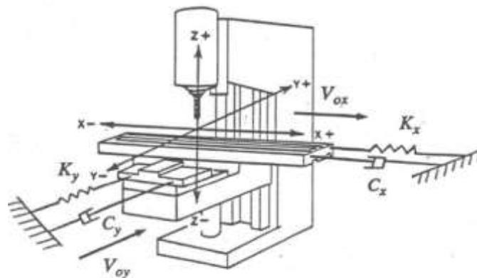
Fig 2: Basis for Mathematical Model of CNC Machine X-Y Tables [3]
