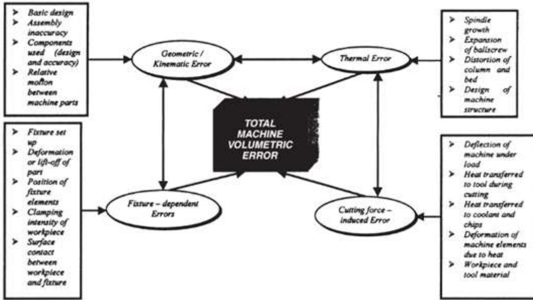
Fig 1: Overview of the error budget in a machine tool and the factors affecting it [1].
