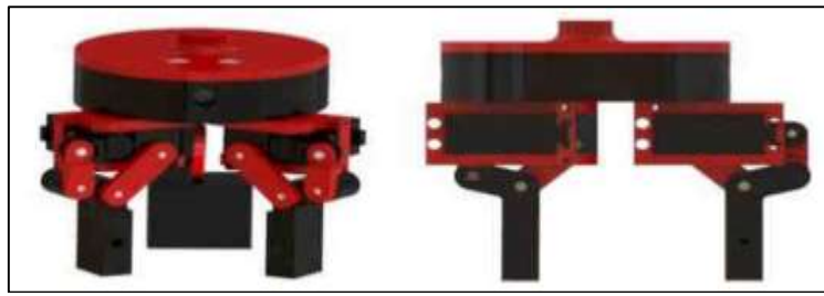
Figure 12: Two modes of gripper (a) 3-finger and (b) 2-finger [ 15 ]
