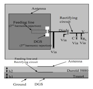
Figure 5: micro-strip antenna used for harmonic rejection
