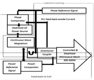
Figure 2: Block Diagram of PACM
