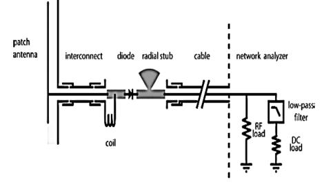
Figure 4: power management circuit of rectenna in electric vehicle.
