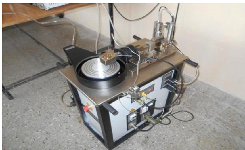
Pin On Disc Setup Specifications of Pin and Disc Tribometer
