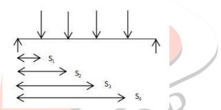
Length of the 1<sup>st</sup> secondary beam  $\ell_{s1} = 5.25$  m Length of the 2<sup>nd</sup> secondary beam  $\ell_{s2} = 5.25$  m Length of the 3<sup>rd</sup>secondary beam  $\ell_{s3} = 5.25$  m Length of the 4<sup>th</sup> secondary beam  $\ell_{s4} = 0$  m
