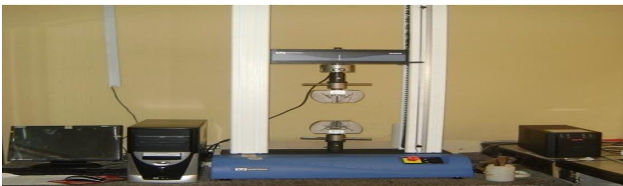
Plate 1: Universal Instron Machine, Model 3369, Maker (Instron)
