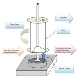
Fig. 4. Working Diagram of maglev Wind Turbine
