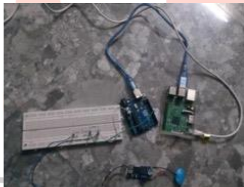
Fig. 6. The battery monitoring system
