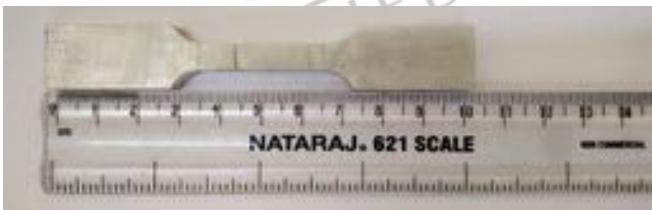
Fig no 4.1: Tensile specimen fracture occur in AA 6082 weld side
