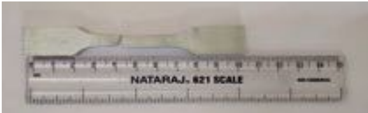
Fig no 4.2: Tensile specimen fracture occur in AA 6082 HAZ
