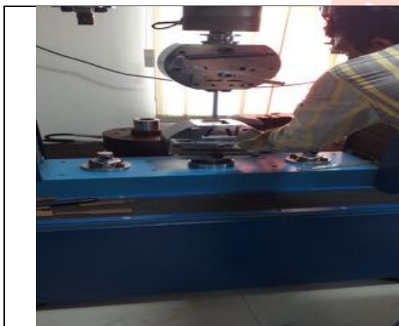
Fig 3 UTM used for tensile and flexural strength
