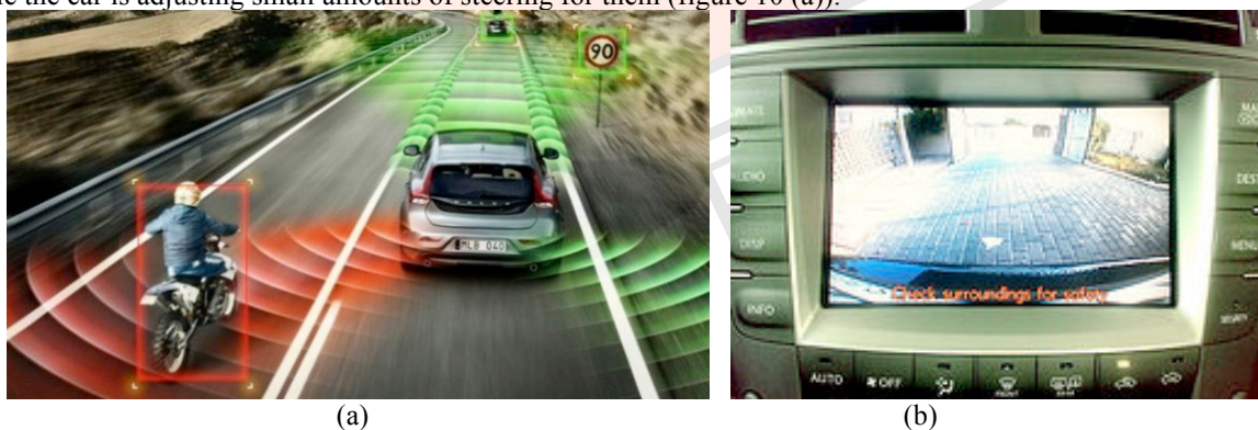
Figure 10: Pictorial representation of the (a) Lane Keeping Assist System (LKA), (b) Parallel Parking Assist.
