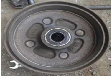
Figure 2.2 used drum for microstructure and Ra value Comparison of thickness of brake drum and lining of new and used brake to find the amount of wear
