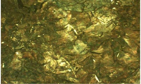
Fig 2.4 Microstructure of brake drum
