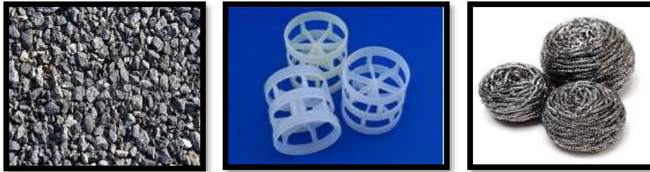
Fig.4 Packing Materials Such As Recycle coarse aggregates, Polypropylene Pall Rings, Steel Scrubber
