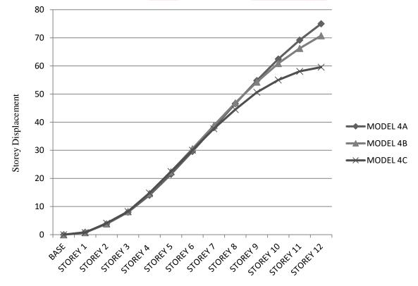
Figure 7. Storey displacement of all models stiffened with both shear wall & RCC X-Bracing system
