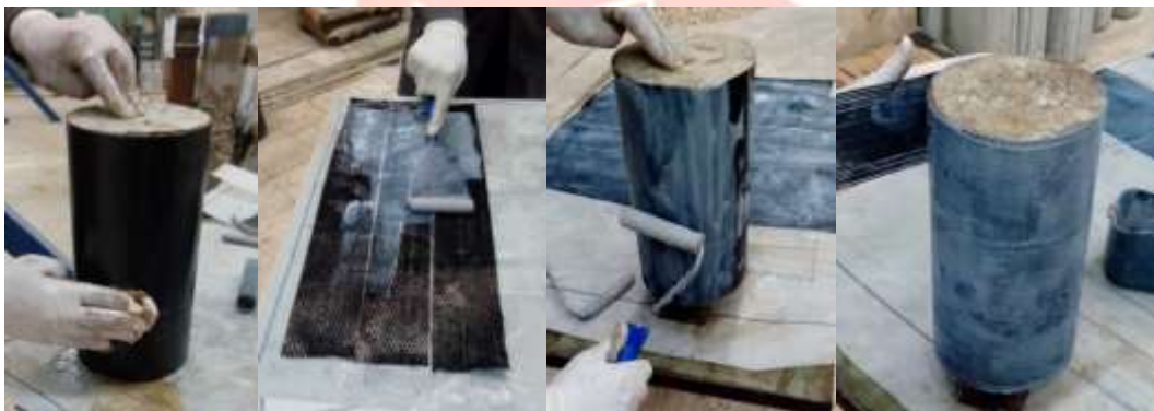
Figure 3. CFRP wrapping using wet layup process
