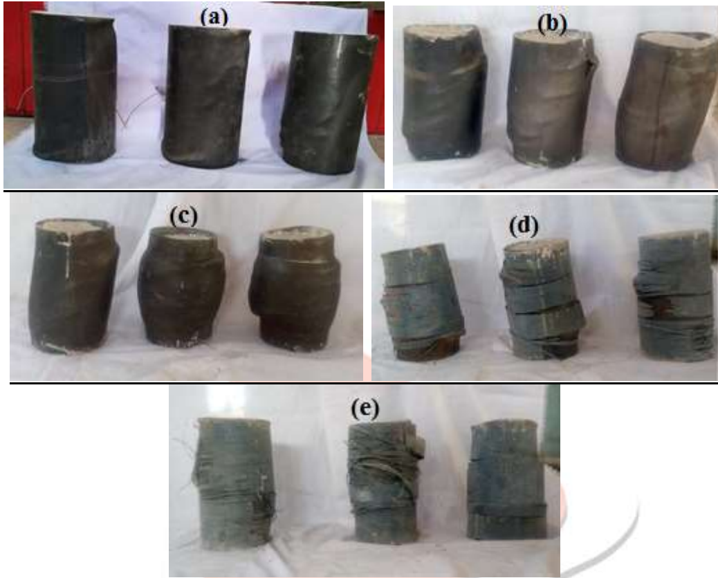
Figure 7. show the failure mode of the specimens. a) Set (1) CFST specimen's t2f0A^* , t2f0B^* , and t2f0C^* . b) Set (2) CFST specimen's t2f0A , t2f0B , and t2f0C . c) Set (3) CFST specimen's t3f0A , t3f0B , and t3f0C . d) Set (4) CFCFST specimen's t2f1A , t2f1B , and t2f1C . e) Set (5) CFCFST specimen's t2f2A , t2f2B , and t2f2C .
