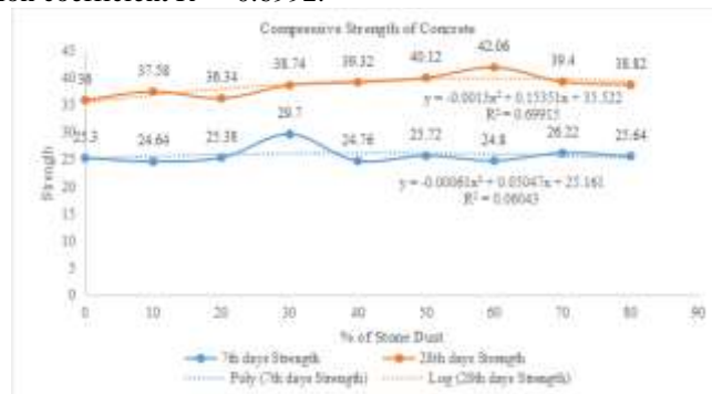
Fig.6: Graphical representation of Compressive Strength of Concrete
