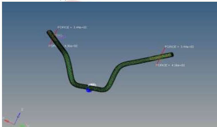
Fig. 3.3 Boundary conditions applied on handle bar
