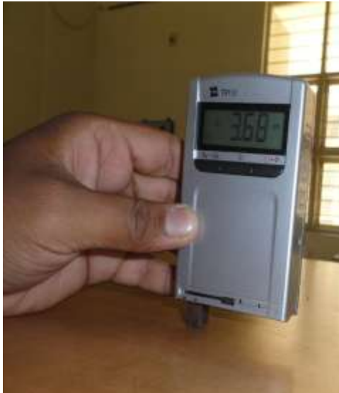
Fig: 2.2 surface roughness TR110
