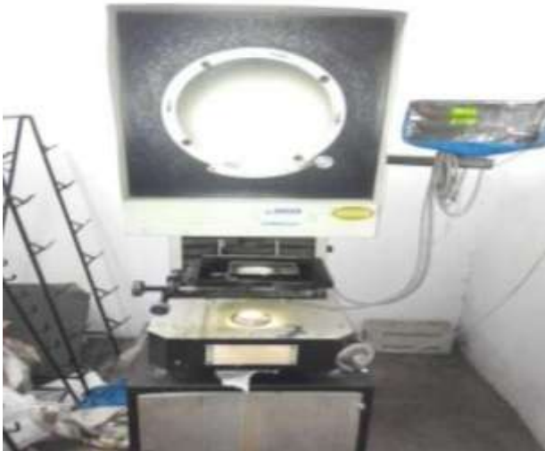
fig 2.3:Profile projector ( at IDTR Jamshedpur)
