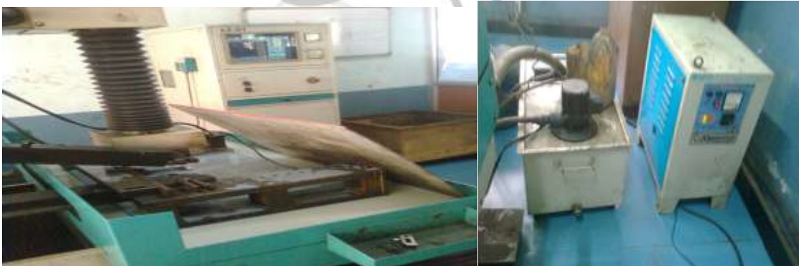
Figure 2.1 Wire cut EDM (at IDTR Jamshedpur) Figure 2.2 WEDM Pulse generator and die-electric fluid
