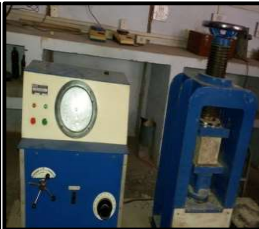
Geopolymer cubes being testing on compressive Strength testing machine
