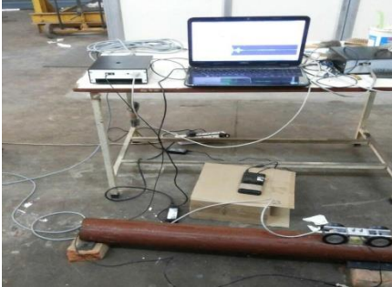
Fig 3.1 Wedge placed at 12 O clock position
