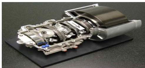
Figure 1: Flywheel for Kinetic energy recovery system of vehicle
