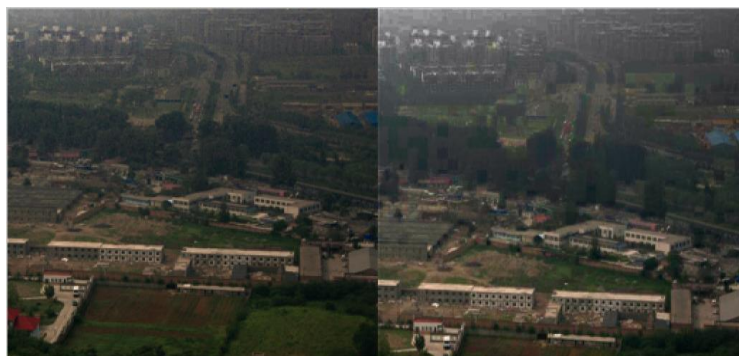
Figure 8 : Image Dehazed using Dark Channel Method
