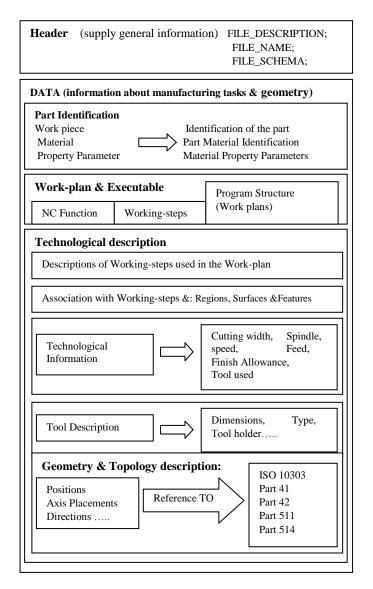
Figure 3- The general structure of a STEP compliant NC code [3].
