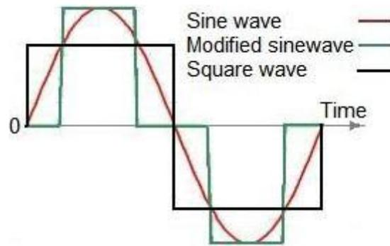
Fig. 4 Sample inverter outputs
