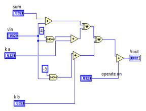
Here 2 separate subVIs are developed for encryption and decryption. Within encryption subVI 2 more subVIs are developed signifying 2 rounds (or 1 cycle) of TEA encryption scheme. Similarly for decryption 2 subVIs within decryption subVI is developed to perform 2 rounds (or 1 cycle) of TEA decryption scheme. Snapshots of front panel and block diagram windows of TEA and its encryption+decryption schemes are as shown in figures below.
