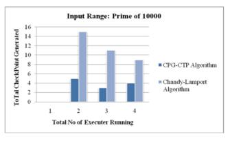
Figure 3 Comparison of checkpoint generation (Input Range: 10000)
