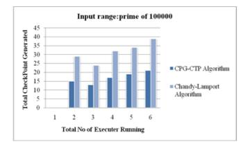
Figure 5 Comparison of checkpoint generation (Input Range: 100000)
