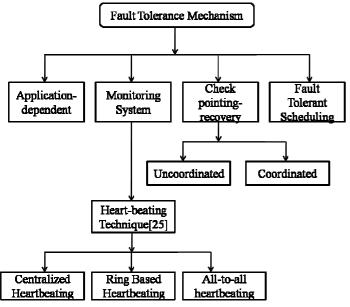
Figure 2 Fault Tolerance Mechanisms
