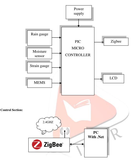
**1.Moisture sensor**: This sensor is used to measure the moisture level and the information is transmitted continuously to the control section and then corresponding values will be displayed
