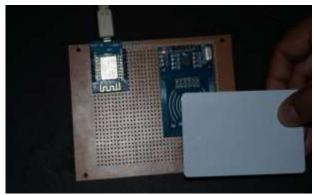
Fig.3 RFID reader scanning the RFID tags
