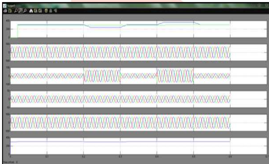
Fig.5 Dynamic performance of DVR with in-phase injection during voltage sag and swell applied to critical load with PI
