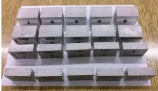
Fig. A: the samples with linear cuts prepared for the measurement of surface roughness
