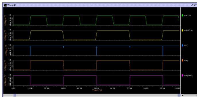
Fig.2(f) Output waveform of The modified pulse triggered flipflop
