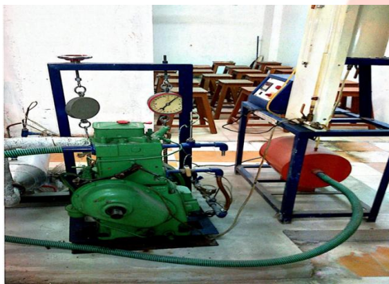
Fig. 2 Single cylinder 4 stroke diesel engine
