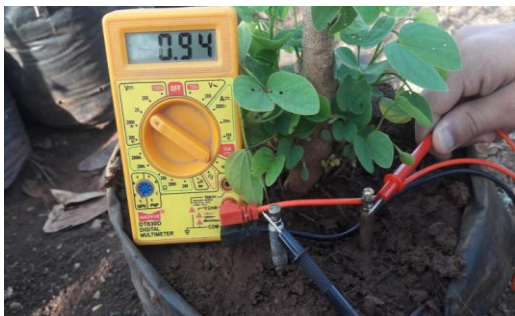
Fig-5: Actual testing on Bauhinia racemosa L. with Cu-Zn pair of electrodes
