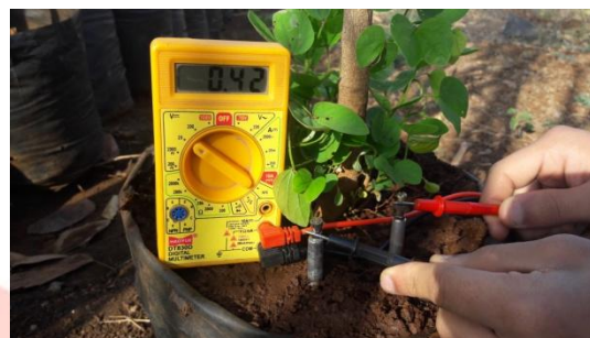
Fig.8: Actual testing on Bauhinia racemosa L. with Zn-Al pair of electrodes
