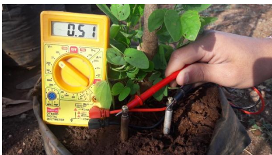
Fig.7: Actual testing on Bauhinia racemosa L. with Cu-Al pair of electrodes
