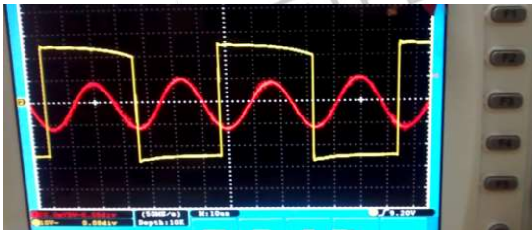
Fig. 8: Second Harmonic Response of Toroid Core Sensor
