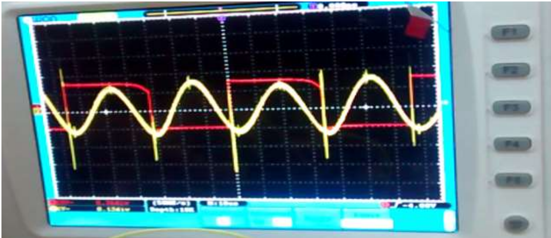
Fig. 9: Second Harmonic Response of PCB based Sensor
