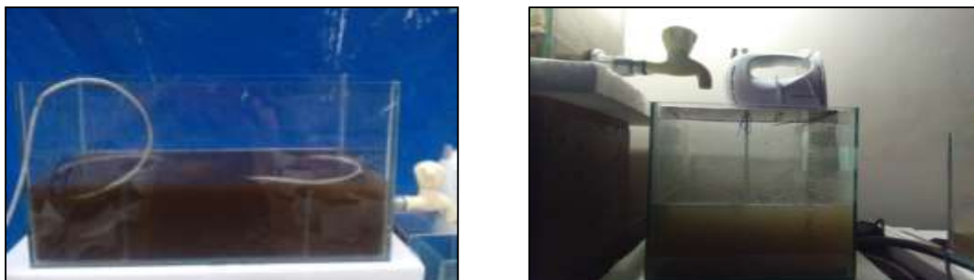
Fig.6 Aeration Tank and Coagulation Tank
