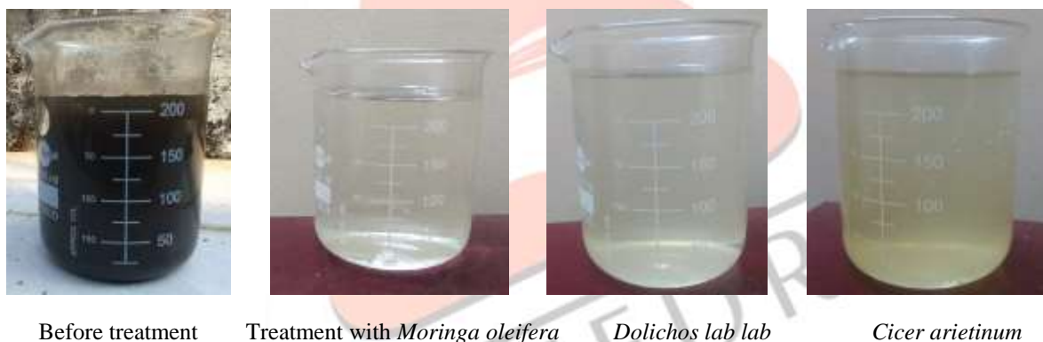
Fig.12 Service station waste water before and after treatment
