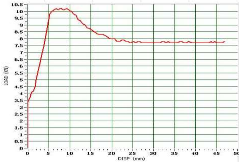
Fig.4 SPECIMEN III-B-BLCS 144 with web holes LOAD VS DISPLACEMENT
