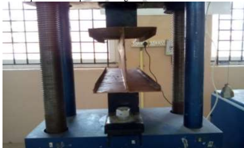
Fig.6 Local buckling occurs at the mid span of the compression flange
