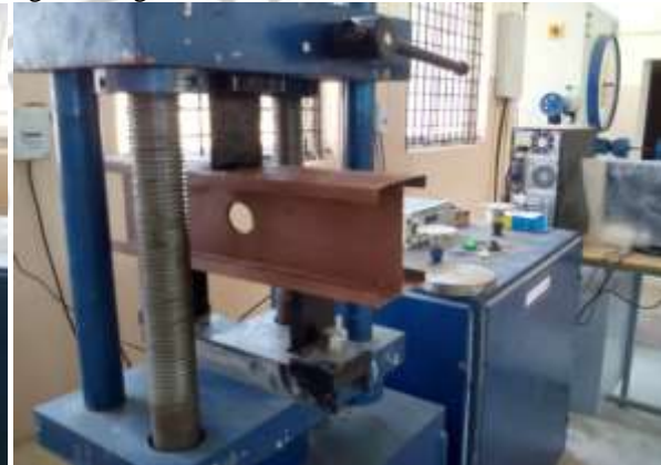
Fig.2 Point loading condition with web holes
