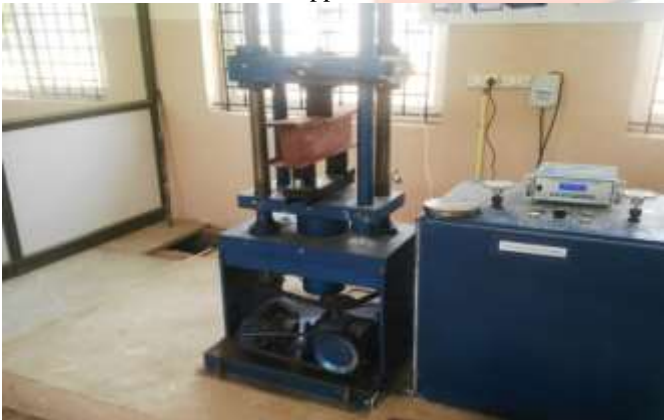
Fig.1 Point loading condition without web holes
